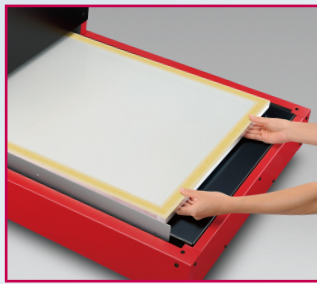
1. Set a screen stretched onto a frame
